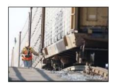
Figure 5: The conductor decoupling cars at the hump.
