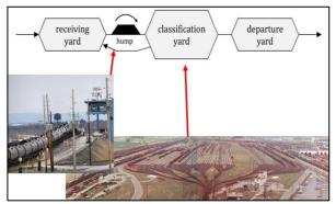
Figure 4: The design of a hump/classification railyard.
